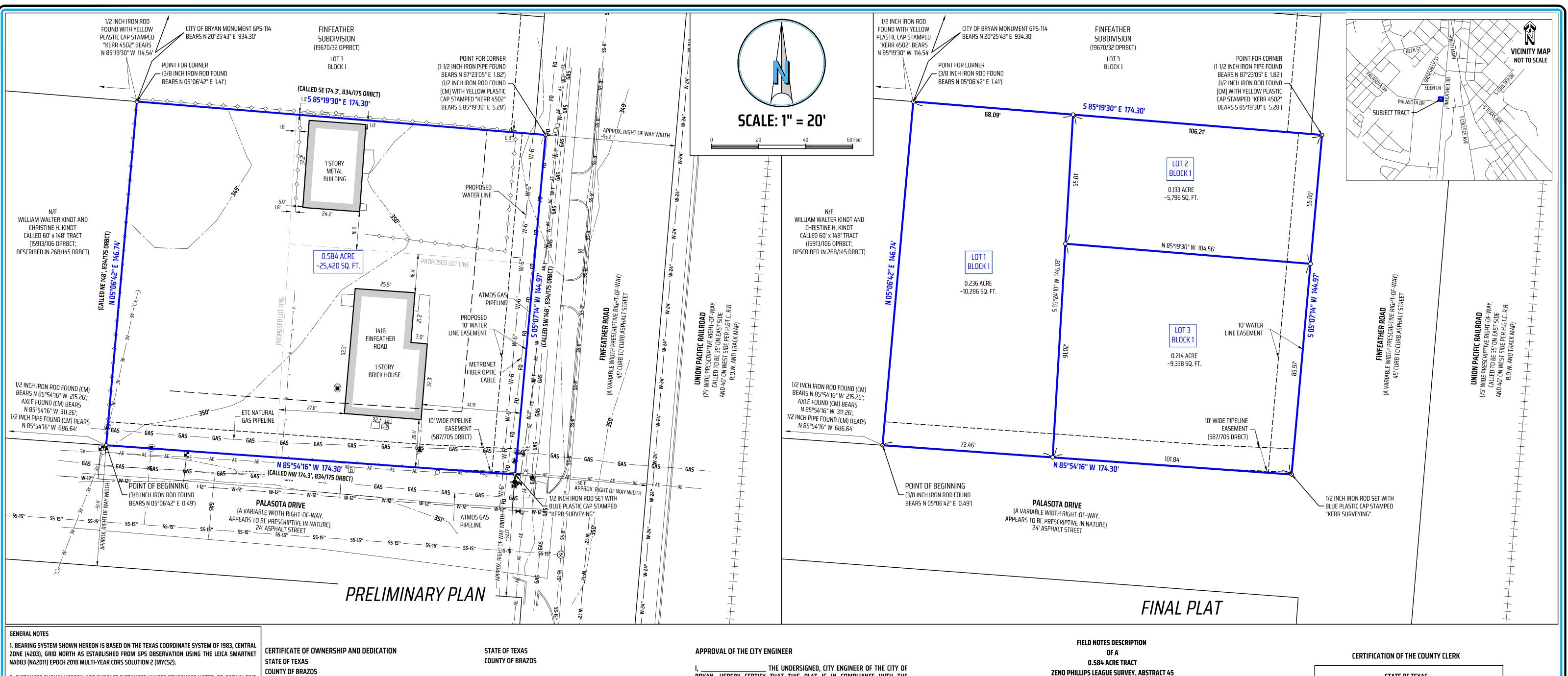
2. DISTANCES SHOWN HEREON ARE SURFACE DISTANCES UNLESS OTHERWISE NOTED. TO OBTAIN GRID DISTANCES (NOT AREAS) DIVIDE BY A COMBINED SCALE FACTOR OF 1.00011309471753 (CALCULATED USING GEOID12B).
